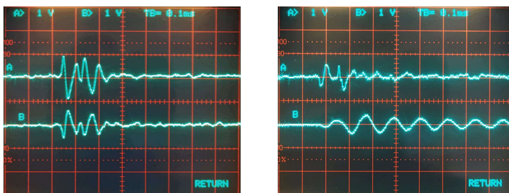
Figure 5: To the left, a signal received by two loop antennas without tuning capacitors, to the right, antenna B is tuned to approximately 10 kHz. This signal cannot be used for time measurement.
